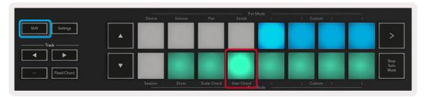
To assign a chord to a pad press and hold the pad and press the notes you want to assign from the keyboard. You can assign up to six notes to each pad. You can input notes with individual key pushes, meaning you do not need to hold down all the notes at once so long as the pad is being held.
