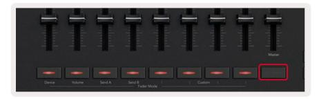
Unlit fader Buttons show no track is associated with that fader channel.
