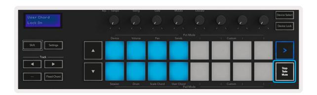
You can use the  $\blacktriangle \blacktriangledown$  buttons to transpose the chord bank in semitones between -12 and +12, any changes show on the screen.
