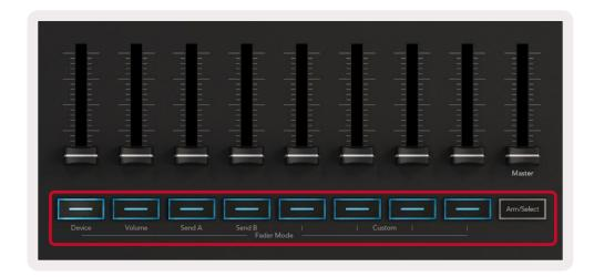
When you move a pot or fader the screen momentarily displays the parameter and its current value. You can assign these modes to either pots or faders at any given time, but both cannot have the same mode.
