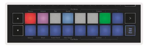
Mute (Yellow) – Press a pad in the bottom row to Mute corresponding tracks. The pads dim for muted tracks, leaving pads for unmuted tracks at their original brightness and colour.
