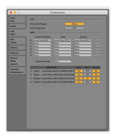
In the Link Tempo MIDI tab you need to copy the settings shown above. Select Launchkey MK3 from the Control Surface menu. Under Input and Output select:
