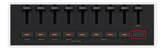
When set to Select the colour of the buttons will match the tracks in Live. Pushing a Fader Button (highlighted blue) will select that track.
