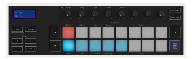
You can toggle between the two Record/Solo modes by pressing Stop/Solo/Mute button. Please note when using Launchkey with Logic Pro X the Stop/Solo/Mute button will only toggle between Solo and Mute modes, there is no Stop mode. The Stop transport button stops playback.
