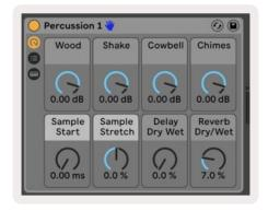
If the Track does not contain a Rack then Device Mode will sync to a selection of eight parameters of the first device. To navigate between devices on a track containing multiple see 'Device Select/Lock'.
