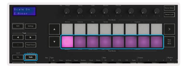
The bottom row of pads light so you can select a scale, the screen shows the selected scale. From left to right the pads select the following scales:
