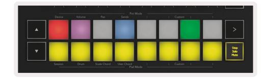
**Clips (Multi-colour**) – the fourth press (after toggling through Stop, Solo and Mute) changes the function of bottom pads to the default Session mode, where the bottom row of pads will again represent clips.
