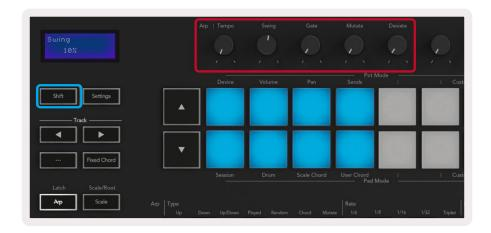
**Tempo –** This pot speeds up or slows down your arpeggio relative to the Arp Rate. Using Launchkey as a standalone controller, this tempo ranges from 60 BPM to 187 BPM. However, when synced with Ableton Live, this pot will have no effect.
